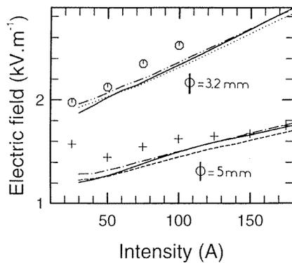
**Figure 8.** Variation of the electric field versus the current intensity for arc diameters of 3.2 mm and 5 mm (experimental and theoretical values). For  $\phi = 3.2$  mm: Schulz-Gulde and Worzyk (1983),  $\circ$ ; SF<sub>6</sub>, —; SF<sub>15</sub>, ·····; SF<sub>15</sub> without radiation absorption, — · — ·. For  $\phi = 5$  mm: Schulz-Gulde and Worzyk (1983), +; SF<sub>6</sub>, —; SF<sub>10</sub>, - - -; SF<sub>10</sub> without radiation absorption, — · — ·.
