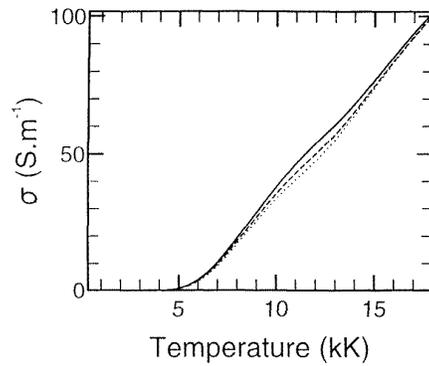
**Figure 1.** Electrical conductivity versus temperature: SF<sub>6</sub>, —; SF<sub>10</sub>, ---; SF<sub>15</sub>, ·····.
