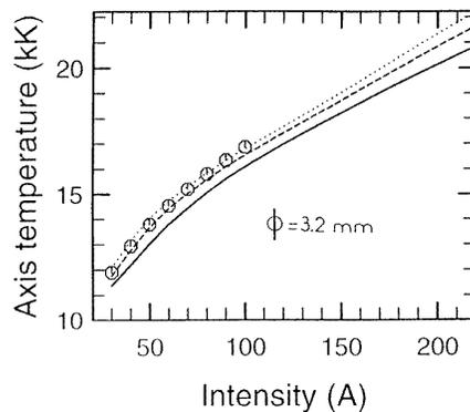
**Figure 7.** Axis temperature versus current intensity for an arc diameter of 3.2 mm (experimental and theoretical values). Schulz-Gulde and Worzyk (1983)  $T(0) = 4455 I \cdot 289$  for  $30 \text{ A} \leq I \leq 100 \text{ A}$ ,  $\circ$ ; SF<sub>6</sub>, —; SF<sub>10</sub>, - - -; SF<sub>15</sub>, ·····.
