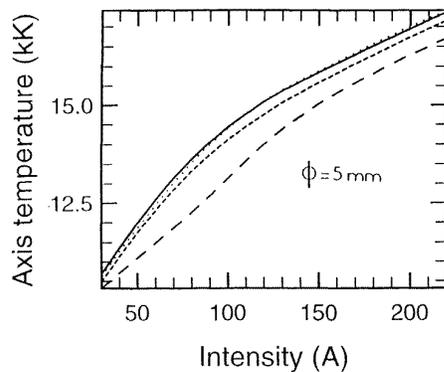
**Figure 5.** Variation of the axis temperature versus the current intensity for an arc diameter of 5 mm. SF<sub>15</sub>, ·····; results with  $\kappa$  of SF<sub>6</sub> and the other functions of SF<sub>15</sub>, ·····; results with  $\sigma$  of SF<sub>6</sub> and the other functions of SF<sub>15</sub>, - - -; results with  $\epsilon$  of SF<sub>6</sub> and the other functions of SF<sub>15</sub>, — · — ·.
