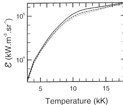
**Figure 3.** Net emission coefficient versus temperature: SF<sub>6</sub>, —; SF<sub>10</sub>, ---; SF<sub>15</sub>, ·····.
