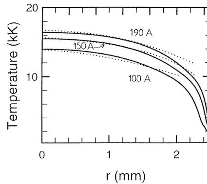
**Figure 6.** Comparison of experimental (· · · · ·) and theoretical (—) radial temperature profile obtained in SF<sub>10</sub> with different current values. Upper curves, 190 A; central curves, 150 A; lower curves, 100 A.
