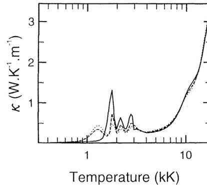
**Figure 2.** Thermal conductivity versus temperature: SF<sub>6</sub>, —; SF<sub>10</sub>, ---; SF<sub>15</sub>, ·····.
