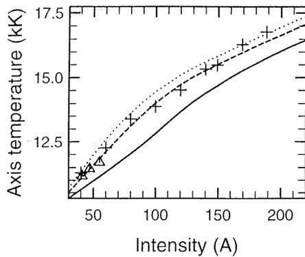
**Figure 4.** Variation of the axis temperature versus the current intensity for an arc diameter of 5 mm—comparison of experimental and theoretical results: Schulz-Gulde and Worzyk (1983), +; Vacquié *et al* (1982),  $\Delta$ ; SF<sub>6</sub>, —; SF<sub>10</sub>, - - -; SF<sub>15</sub>, ·····.
